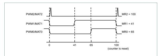
Fig 78. Sample PWM waveforms with a PWM cycle length of 100 (selected by MR3) and MAT3:0 enabled as PWM outputs by the PWCON register.
