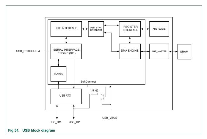
The USB Device Controller has a built-in analog transceiver (ATX). The USB ATX sends/receives the bi-directional USB\_DP and USB\_DM signals of the USB bus.
