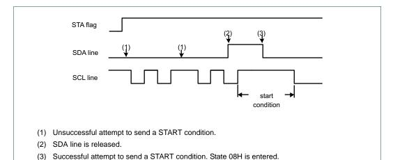
Fig 43. Recovering from a bus obstruction caused by a LOW level on SDA
