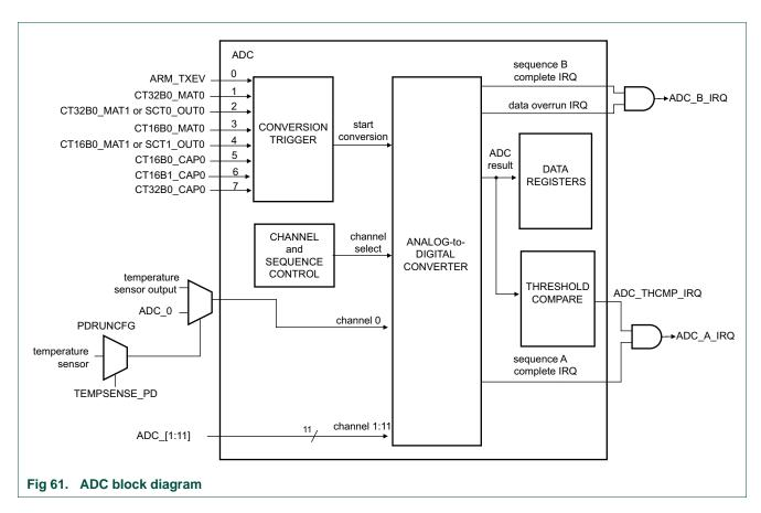
The ADC controller provides great flexibility in launching and controlling sequences of A/D conversions using the associated 12-bit, successive approximation A/D converter. A/D conversion sequences can be initiated under software control or in response to a selected hardware trigger. The ADC supports eight hardware triggers.
