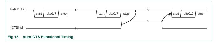
During transmission of the second character the  $\overline{\text{CTS}}$  signal is negated. The third character is not sent thereafter. The USART maintains 1 on TXD as long as  $\overline{\text{CTS}}$  is negated (high). As soon as  $\overline{\text{CTS}}$  is asserted, transmission resumes and a start bit is sent followed by the data bits of the next character.
