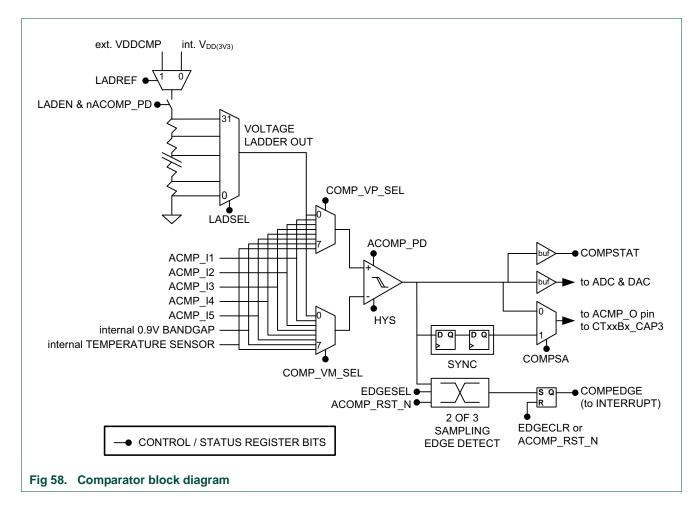
The comparator has 8 inputs multiplexed separately to its positive and negative inputs. The multiplexers are controlled by the comparator register CTL (see <u>Figure 58</u> and <u>Table 210</u>).
