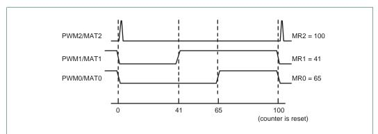
Fig 47. Sample PWM waveforms with a PWM cycle length of 100 (selected by MR2) and MAT1:0 enabled as PWM outputs by the PWMC register.
