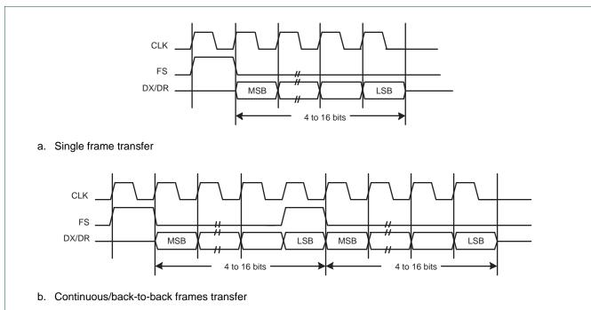
Fig 35. Texas Instruments Synchronous Serial Frame Format: a) Single and b) Continuous/back-to-back Two Frames Transfer
