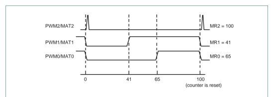
Fig 43. Sample PWM waveforms with a PWM cycle length of 100 (selected by MR2) and MAT1:0 enabled as PWM outputs by the PWMC register.
