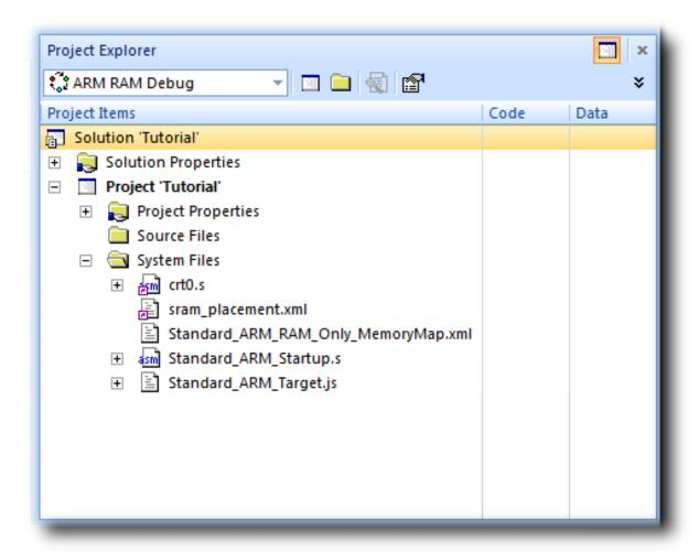
The project name is shown in bold to indicate it is the active project (and, in our case, the only project). If you have more than one project, you can set the active project by using the drop-down box on the **Build** tool bar or by right-clicking the desired project's name in the **Project Explorer** to display the shortcut menu with the **Set as Active Project** command.
