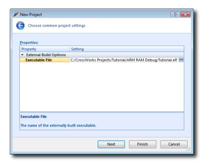
In the Executable File field, type the path to the Tutorial.elf executable file we generated earlier. For example, if the project was created in the C:/CrossWorks Projects/Tutorial directory and was built using the ARM RAM Debug configuration, the path to the executable file will be C:/CrossWorks Projects/Tutorial/ARM RAM Debug/Tutorial.elf.
